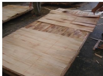
Overlaying with veneer
